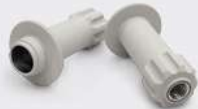
PEO coating on Top pulley
